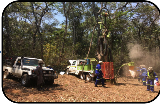
2. Shallow Aircore Drilling sample bedrock below the sand.
