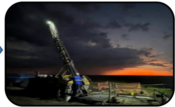
4. Core Drilling is used to follow-up on copper anomalies.
